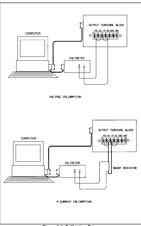
Figure A-1. Calibration Setup
